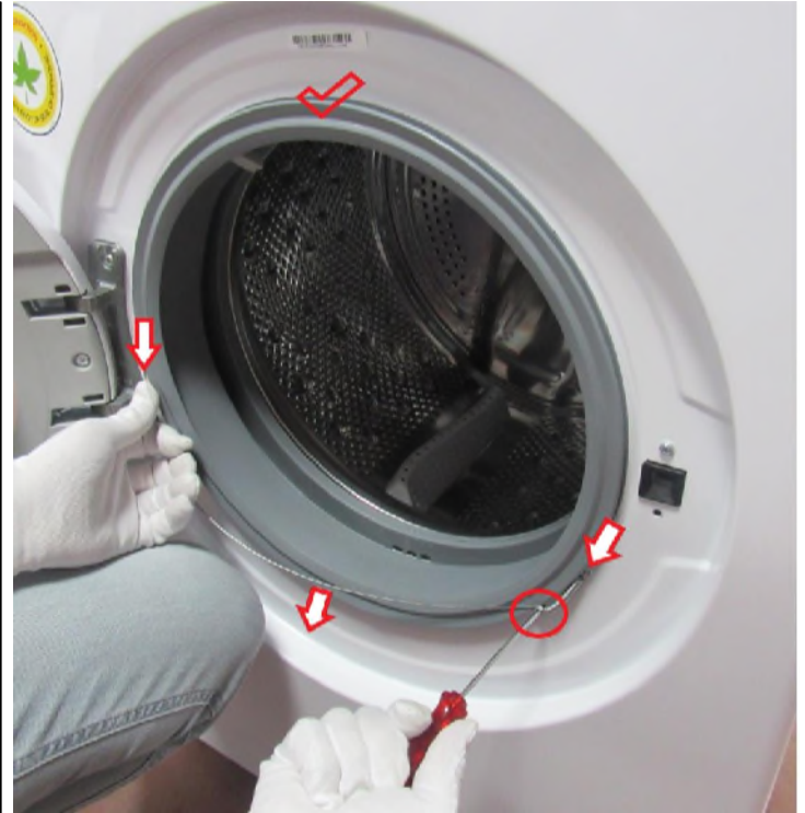
4.3 Fix the tub bellow seal and fix the wire by using the small screwdriver
