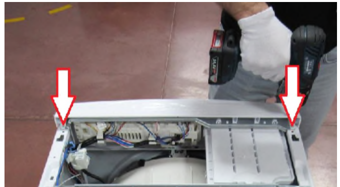
4.12 Tighten two screws fixing control panel.
