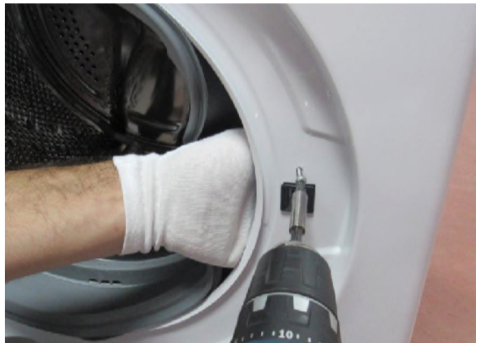
4.6 Tighten the door lock screw
