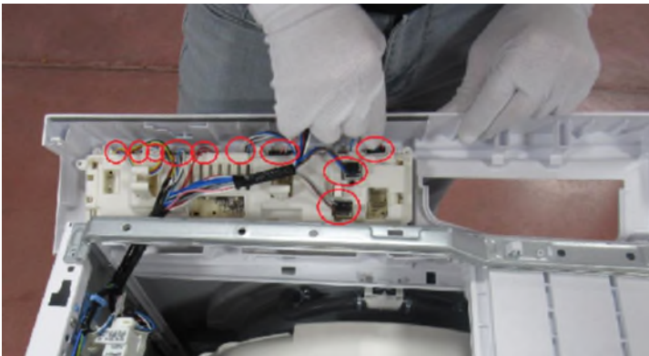
3.6 Remove the sockets on the card.
