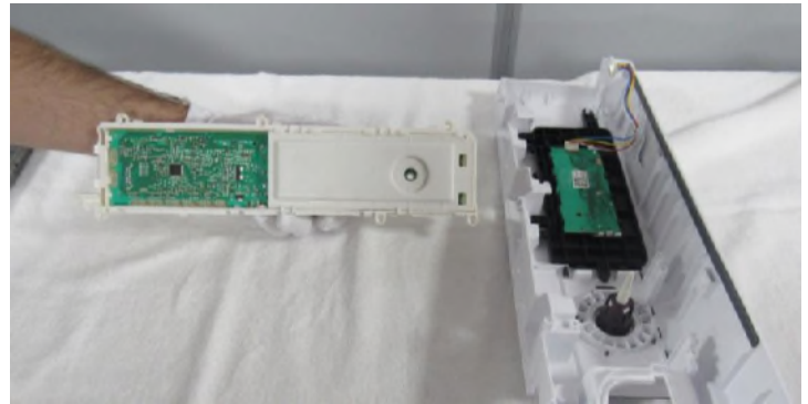
3.8 After releasing sockets, remove PCB box from its housing
