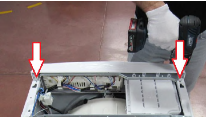
4.4 Tighten the two screws on control panel.
