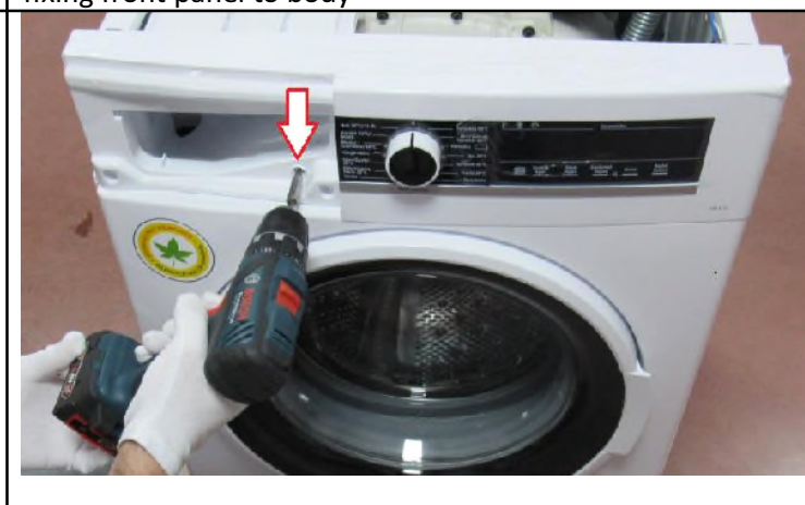
3.11. Tighten the screw which fixes the control panel to the front panel.
